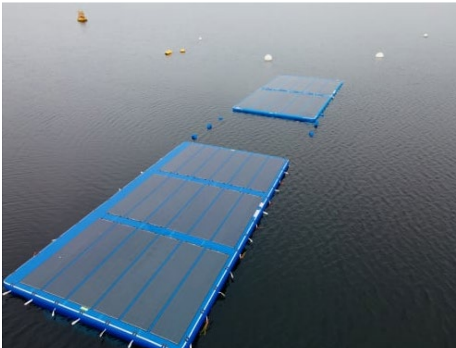
Figure 9: Application of flexible semi-fabricates in field of Floating PV. Prototype from project Solar@Sea [8].
