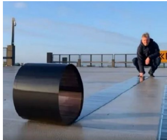
Figure 6: Left: In 2020, for the 9.2 meter long laminate in the STAL-project, manual stitching was still needed. Right: In 2022, a 10 meter long laminate has been produced without stitching.
